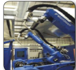
**RHINO WRAP™ Weld Shield Sleeve** protecting a hydraulic hose on a robotic welding arm
