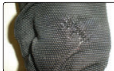
Close up of RHINO SLEEVE® HT sleeving after pin hole burst
