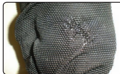
Close up of RHINO SLEEVE® HT sleeving after pin hole burst
