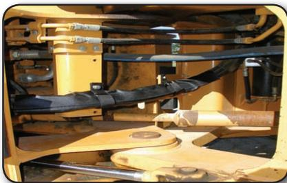
**RHINO HANGING STRAPS™** are held in place by the 3/8" (9.5mm) grommet. Mounting can be vertical or horizontal. The hook & loop used in our hanging straps are a special product designed for military and industrial applications.
